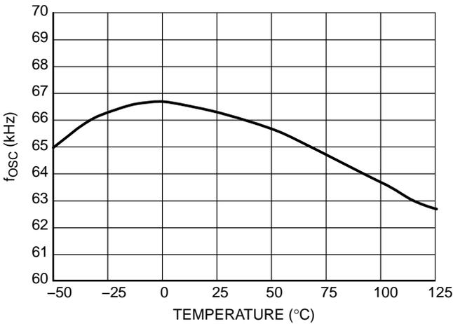
Figure 13. Oscillator Frequency  $f_{\text{osc}}$  for the 65 kHz version
