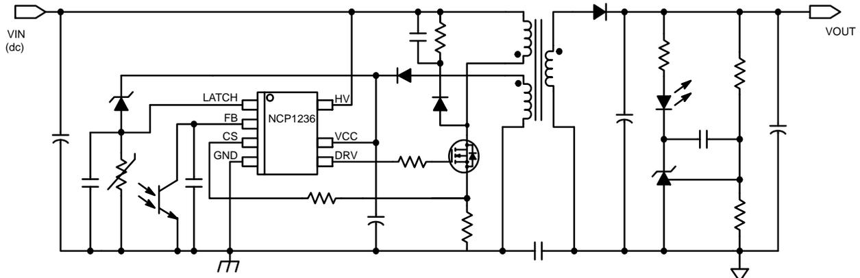
Figure 1. Flyback Converter Application Using the NCP1236
