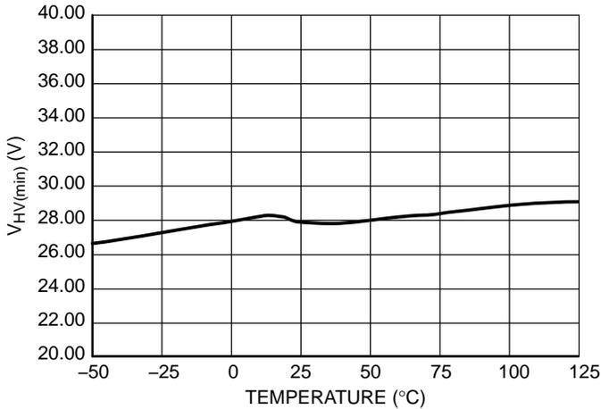
Figure 3. Minimum Current Source Operation
