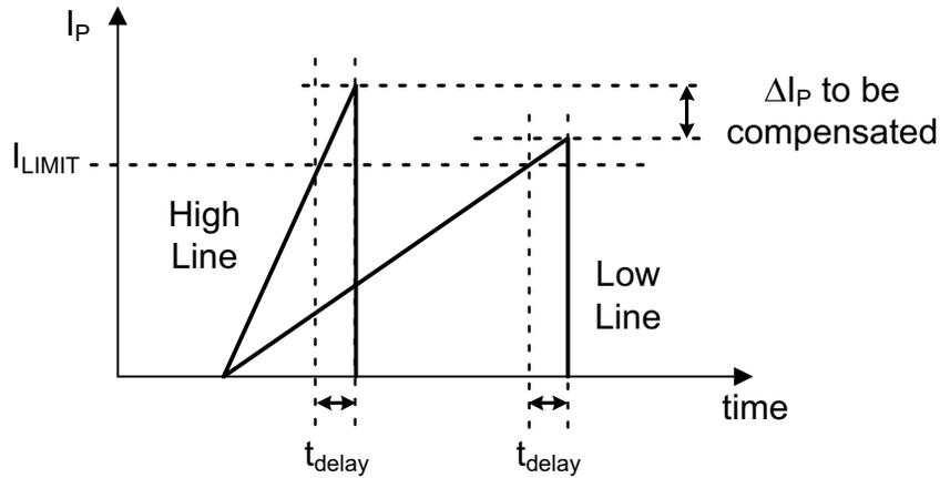
Figure 38. Line Compensation for True Overpower Protection
