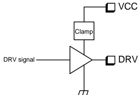
Figure 35. Clamped Driver
