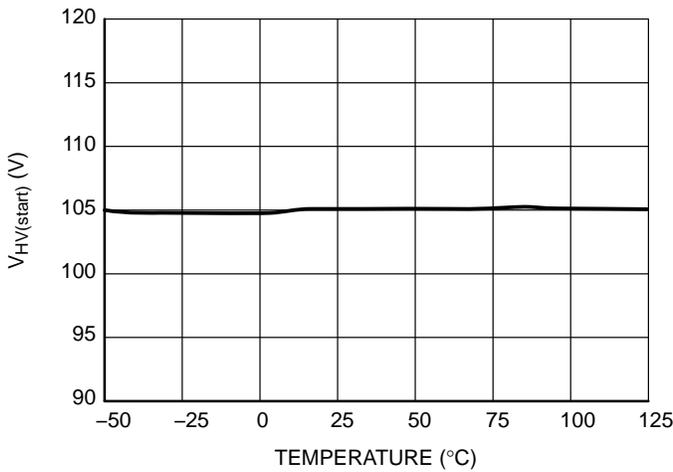
Figure 5. Brown-out Device Start Threshold
