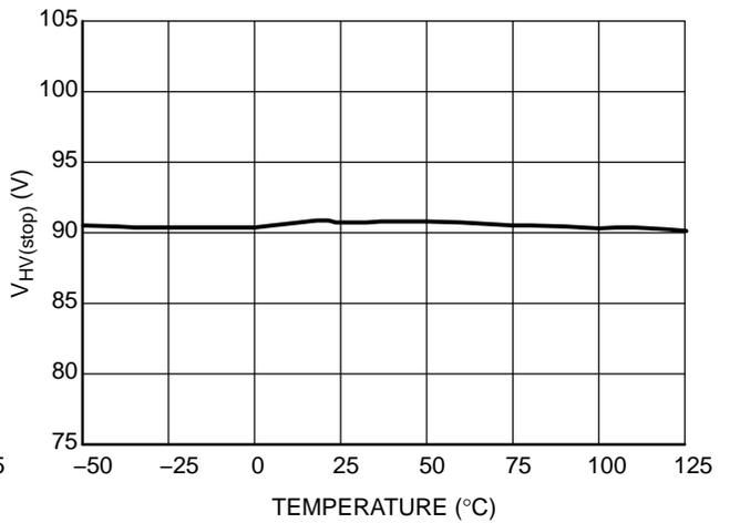
Figure 6. Brown-out Device Stop Threshold
