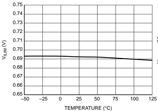
Figure 7. Maximum Internal Current Setpoint
