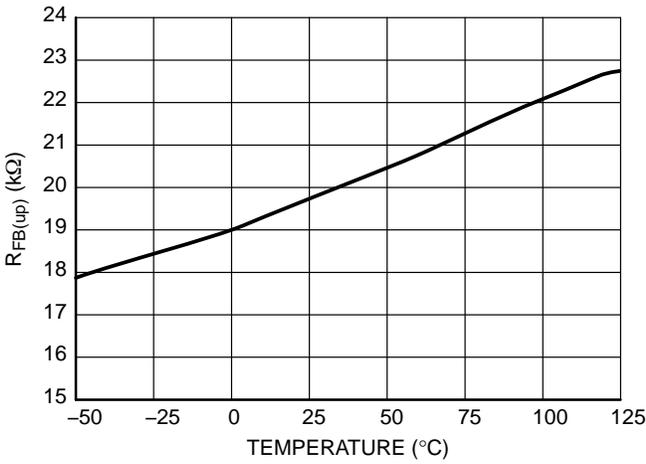
Figure 11. FB Pin Internal Pull-up Resistor  $R_{\text{FB(up)}}$
