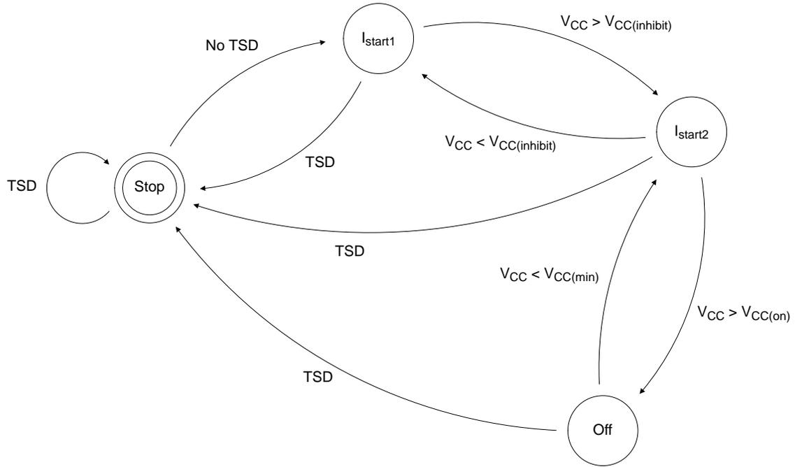
Figure 52. HV Start-up Current Source State Diagram
