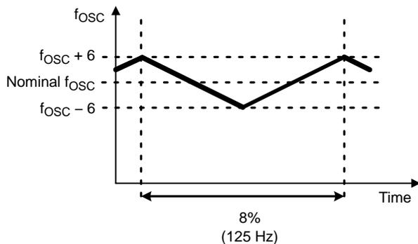
Figure 34. Frequency Jittering
