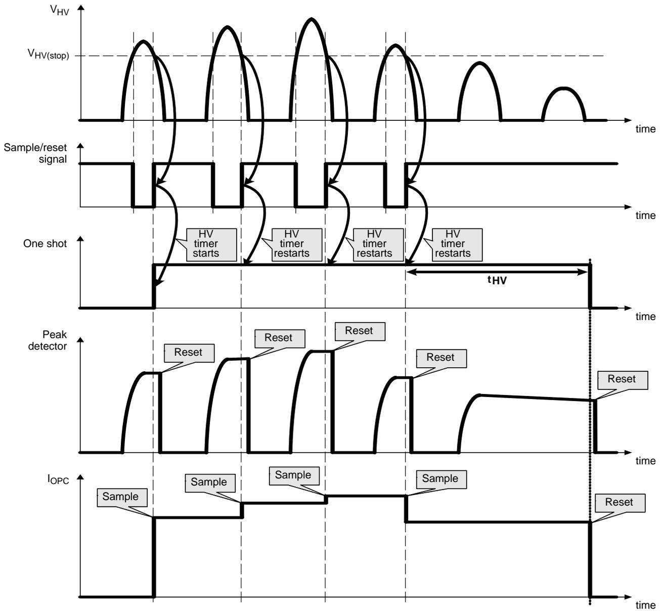
Figure 41. Overpower Compensation
