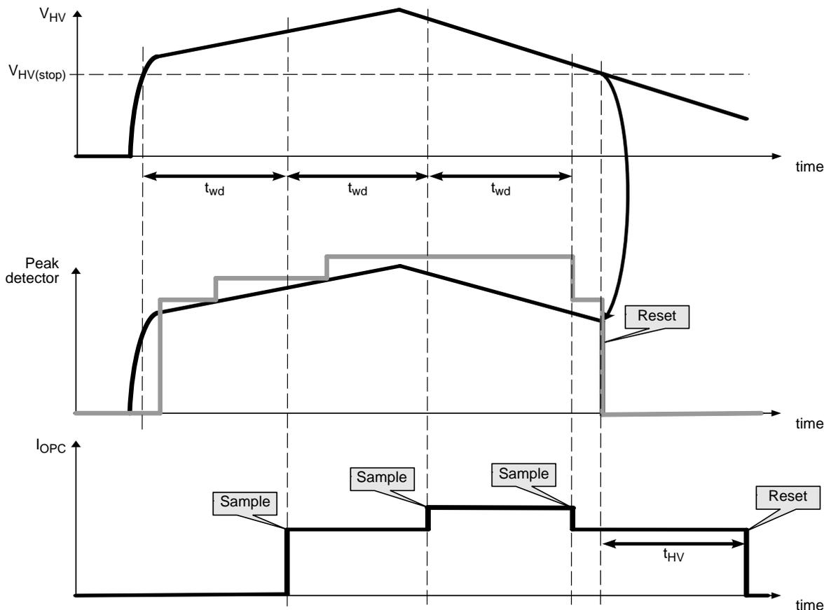
**Figure 42. Overpower Compensation**
